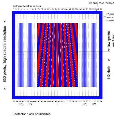
Figure 2. Layout of the MATISSE beams on the Aquarius detector. In the middle, interferometric fringes are encoded in horizontal direction. The four photometric channels are located pairwise at the left and right of the detector. Spectral dispersion is in the vertical direction.
