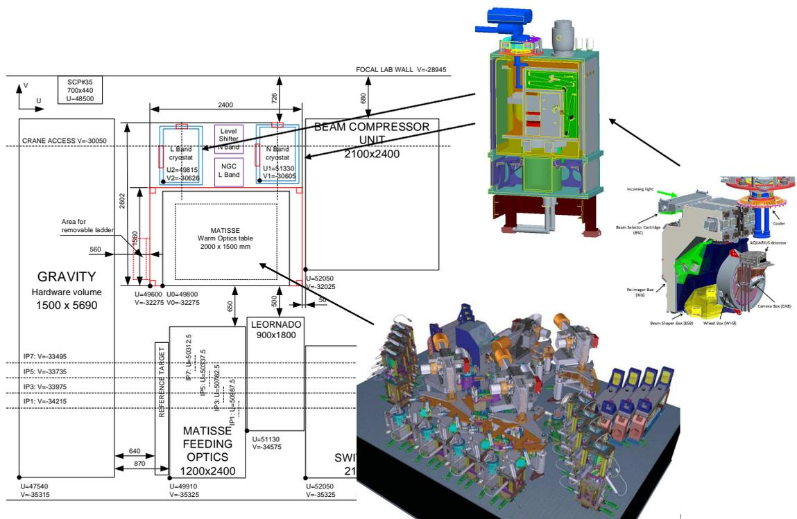
Figure 3. Future location of MATISSE in the VLTI laboratory. One can see the Warm OPTics table and the two cryostats above. This location is currently used by MIDI. a) The MATISSE Warm OPTics table with its optical components. b) One of the two MATISSE cryostats, which holds the Cold Optics Bench and the detector. c) The MATISSE Cold Optics Bench with its subsystems.
