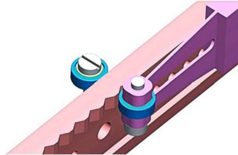
Figure 8: Slit slider indent positioning principle
