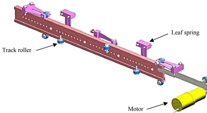
Figure 7: Slit slider mechanisms showing the general mechanism principle; 5 accurately positioned ball bearings that act as track rollers with 5 additional spring loaded bearings positioned opposite these 5 track rollers and a motor attached to the carriage to allow a sliding motion.
