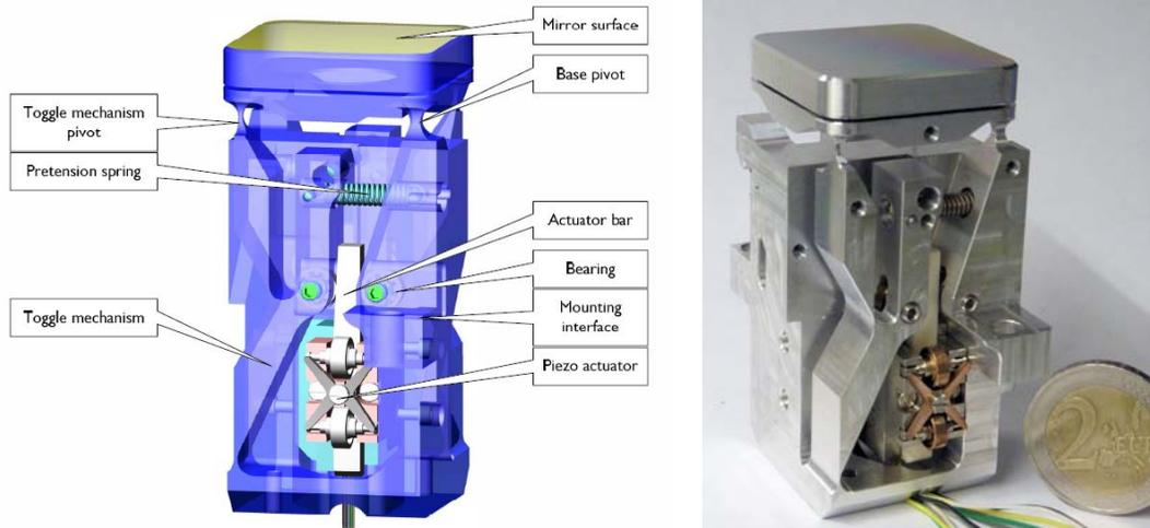
Figure 10 Tip-Tilt Mechanism including piezo motors
