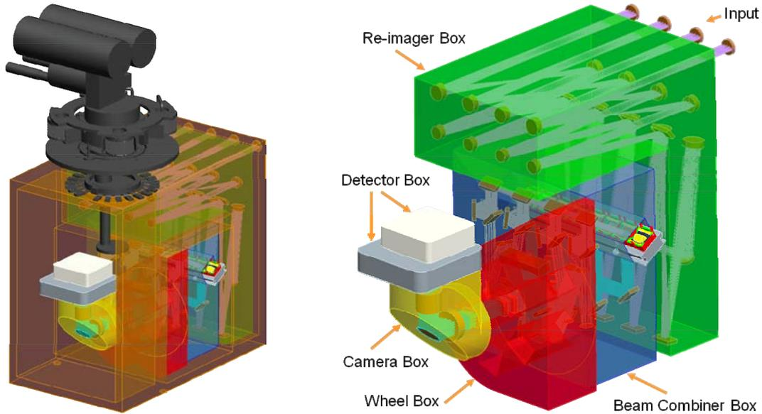
Figure 3: Modular division of the GMA COB concept, backbone and cooler not shown (right)
