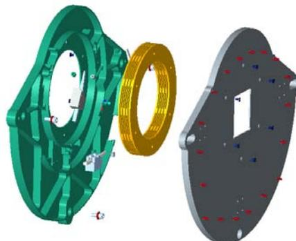
Figure 13: NOVA-ASTRON piezo driven tip/tilt/focus unit
