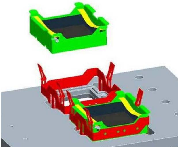
Figure 11: Mirror clip design, in the air the optical element assembled into the mirror cell by means of leaf springs, at the front in fully assembled state
