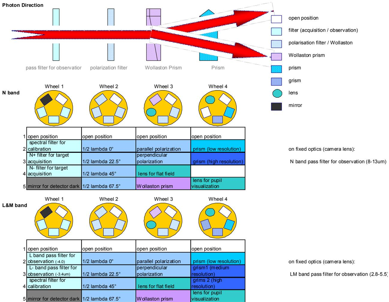
Figure 12: The wheel box contains 4 wheels with 5 optical components each.
