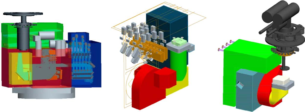
Figure 2: The three MATISSE recombination concepts side by side (at random colouring). The Pair-Wise concept with PI-shifter; PW-PI (Left), the Pair-Wise recombination without PI-shifter; PW (Centre) and the Global Multi-Axial concept; GMA (Right).
