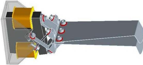
The shutter has two purposes: a light blocking function and a high speed shutter for detector remanence analysis. Providing both functionalities within one mechanism proved impossible so two shutters will be provided. The Cold Shutter is a slow and relative simple type. An off the shelf warm fast shutter is placed just before the entrance window, the side facing the cryostat is gold coated to let the detector look back into the cold environment during a remanence test.
