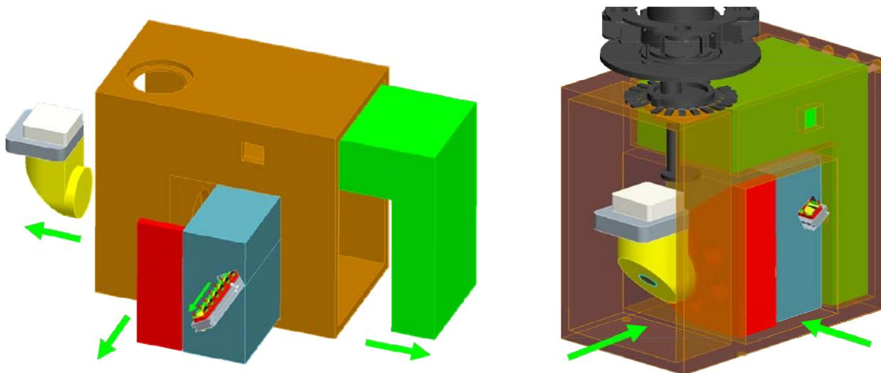
Figure 5: Left: module removal (arrows indicate slide direction). Left: Wheel Box and Beam Combiner Box will be stacked as one unit. The Re-imager Box is only removable when the whole upper part of the cryostat is removed. However, Re-imager mechanisms will be removable as a cartridge just like the Photometric mechanism. Right: the two access sides for maintenance once operational.
