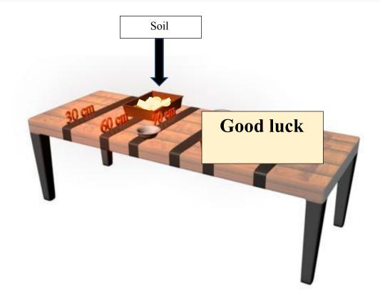
Representation of a long table with two strategic locations for the shovel arm challenge. The goal is to use a student-designed robotic arm to move dirt / sand from the rectangular container (60cm line) to a container placed at the 70cm line without any part of the body sticking out the line of 30 cm.
